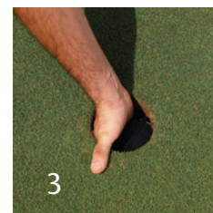
Gently push sensor prongs into hole wall
