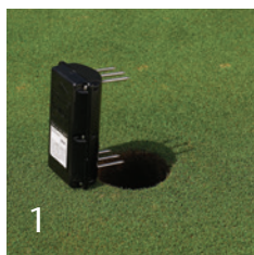
Cut hole using standard cup cutting tool
