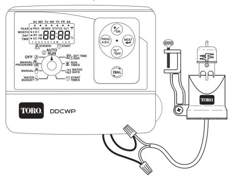
The DDCWP will respond to a Toro, TRS wired Rain Sensor™. Cut the yellow looped wire from the controller, and using waterproof connectors, connect the two wires from the rain sensor to either ends of the yellow controller wires.
