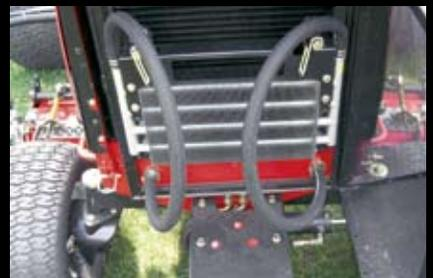
The hinged radiator screen and tip-out oil cooler provide quick and easy access for cleaning.
