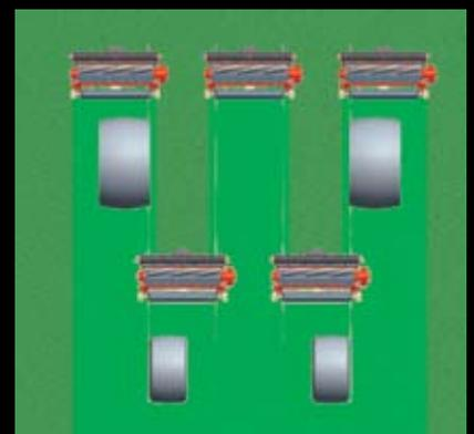
The wheel alignment eliminates the distinct tyre tracks and intermediate stripe for a more visually appealing finish.
