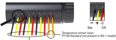
Configurable acquisition inputs (3 inputs for MS-4 model, 1 input for MS-1 model)
